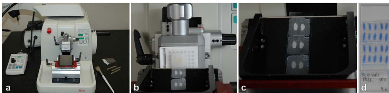
Figure 1. Collection of intact rice kernel sections with Scotch packaging tape. Leica RM2265 rotary microtome with paraffin block containing rice kernels clamped in the microtome chuck (a). Collecting sequential, longitudinal sections of rice kernels (b and c). Slide showing two stained sections collected from a paraffin block containing 10 whole, milled rice kernels (d).
